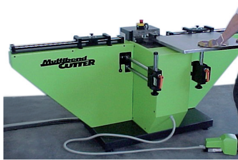
MBC-Cutter (optional) As Auxiliary Unit to cut holes, shapes and forms after corner forming
